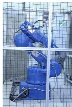
**Fig.6 Coating Robot**
